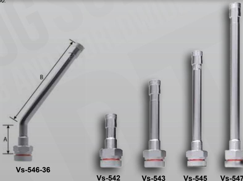
Install the valve with care and do not over-torque: the recommended torque is 7 to 10 Ft-Lb (9 to 16 Nm.)
