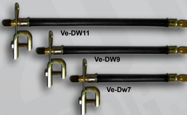
Recreational Vehicle Dual Wheel Extension with flexible hose. Provides easy access to the inner rear tire on campers, recreational vehicles and light trucks. Also useful for fitting to spare wheels that are often difficult to access when checking the pressure. Fits standard valve cap threads. Clamp is easily secured to rim cut out.
